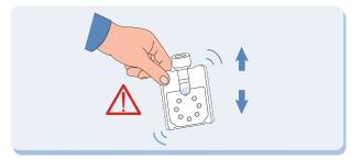
7.Open the cabin door of Integrated Nucleic Acid Testing Device, and insert the Reaction Card into the device according to the direction indicated on the Anaplasma/Ehrlichia Reaction Card, and push it to the fixed position of the bottom card slot, close the cabin door.
