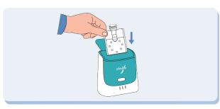
9. Press start button on the software to start the run. The light is flashing blue during the operation.
