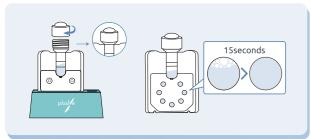
5.Firmly press the protruding arc-shaped air bag on the sample tube cap of the Reaction Card to deform it and recess it into the tube.
