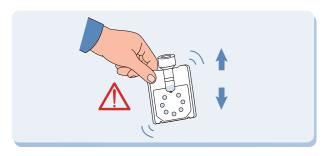
7.Open the cabin door of Integrated Nucleic Acid Testing Device, and insert the Reaction Card into the device according to the direction indicated on the Reaction Card, and push it to the fixed position of the bottom card slot, close the cabin door.
