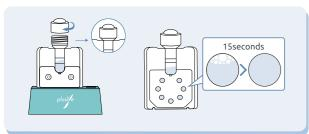
5.Firmly press the protruding arc-shaped air bag on the sample tube cap of the Reaction Card to deform it and recess it into the tube.
