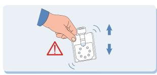
7.Open the cabin door of Integrated Nucleic Acid Testing Device, and insert the Reaction Card into the device according to the direction indicated on the Babesia Reaction Card, and push it to the fixed position of the bottom card slot, close the cabin door.
