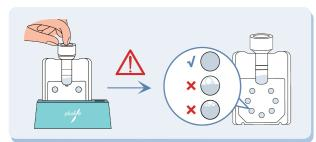
6. Hold the card, shake it up and down for 10 times in about 5 seconds. Then proceed to next step immediately.
